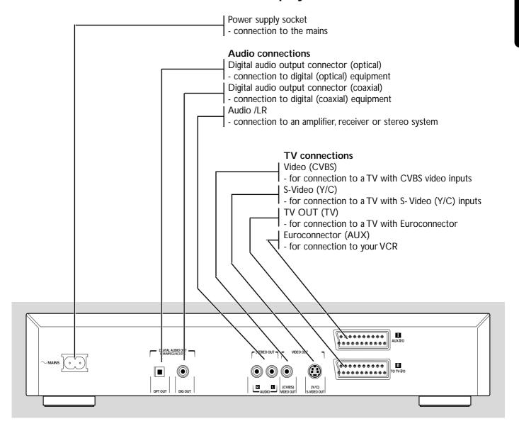
Caution: Do not touch the inner pins of rear panel connectors. Electrostatic discharge may cause permanent damage to the unit.
